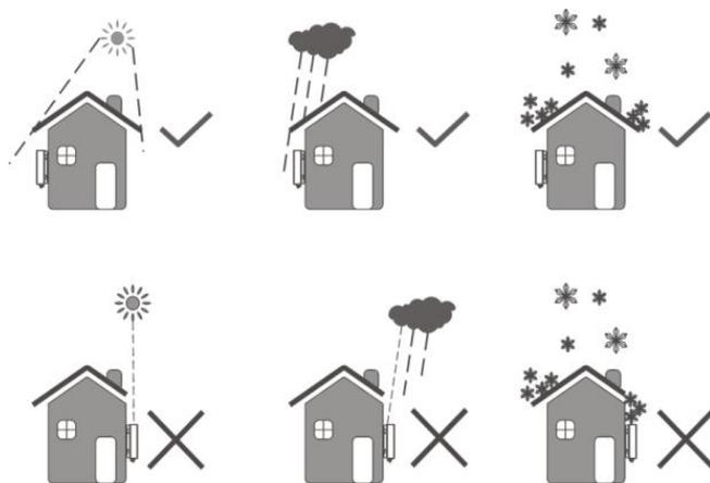
FIG.6-1 Inverter Installation Positions
