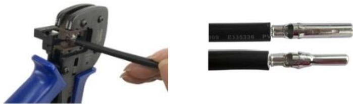
FIG. 7-12 Crimp the Contact
