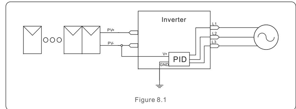
The integrated Anti-PID module repairs the PID effect of the PV model at night. When operating, the inverter LCD screen displays "PID-repairing" information, and the red light is on. The Anti-PID function is always ON when AC is applied.
