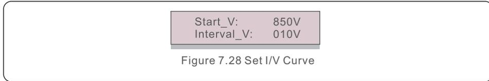
Start\_V: The start voltage of the I/V scan. (Adjustable from 850V-1000V)
