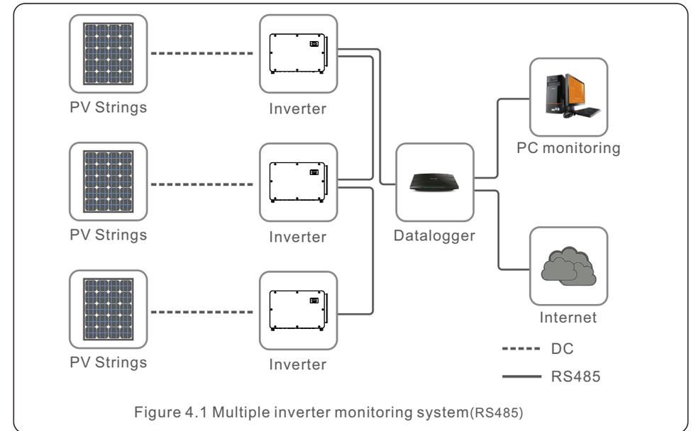
Figure 4.1 Multiple inverter monitoring system(RS485)
