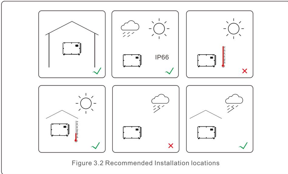
Figure 3.2 Recommended Installation locations
