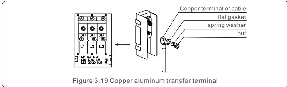
Figure 3.19 Copper aluminum transfer terminal
