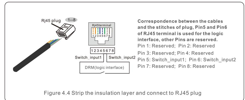
3.Connect RJ45 to DRM (logic interface) .
