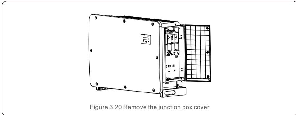
Figure 3.20 Remove the junction box cover
