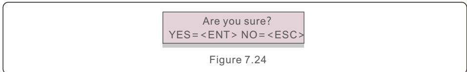
Fan Test is a factory test function. Press the ENTER key to start the test.
