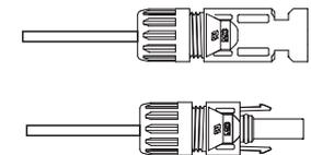
Figure 3.15 Connector with Cap nut Screwed on
