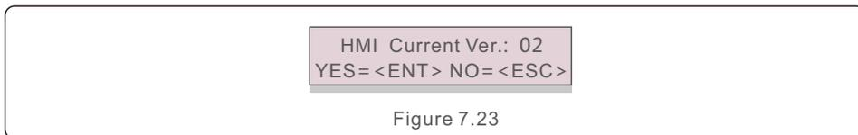
Updater is for updating LCD firmware. Press the ENTER key to start the process.
