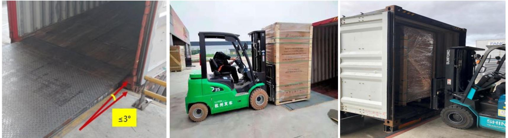
Container bottom level and the loading/ unloading platform level must be at the same level, and the inclination angle must be  $\leq 3^\circ$ .
