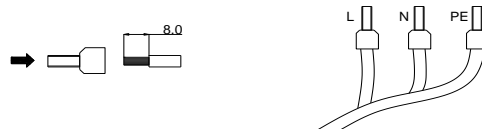
FIG. 7-8 Crimp the Three-core's Ferrule
