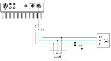
Note: The arrow has to be pointing to the grid side, not the load side.
