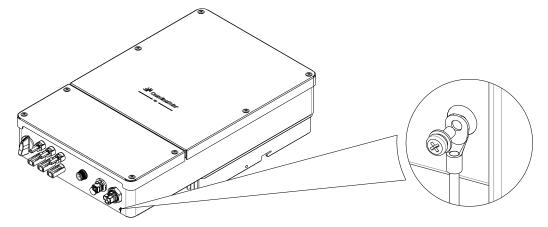
FIG. 7-1 External Grounding Point Position
