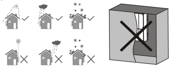
FIG.6-1 Inverter Installation Positions
