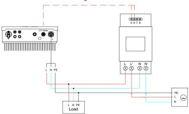
FIG.2 Electrical and Signal Connection Diagram
