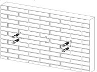
FIG.6-7 Install Expansion Anchors
