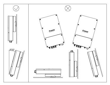
FIG.6-5 Installation Angle Requirements
