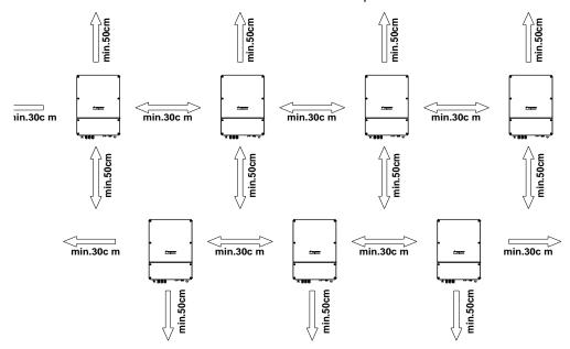
FIG.6-4 Staggered Installation Mode (Recommended)
