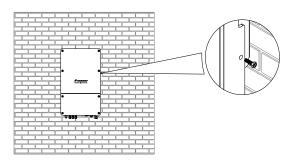
FIG. 6-10 Fix Both Sides of Inverter
