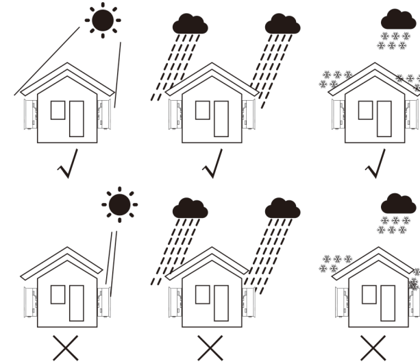
Figure 5.1 Recommended Installation locations
