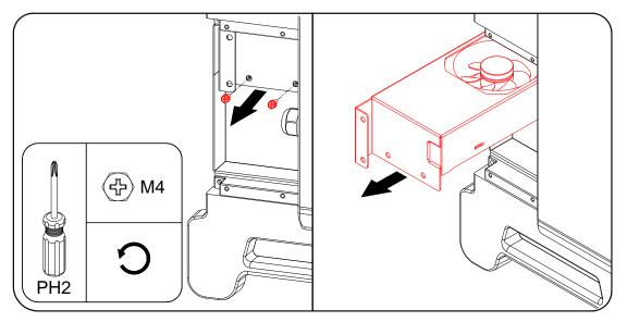
Insert the fan connector into the track, and secure the fan connector by screws.
