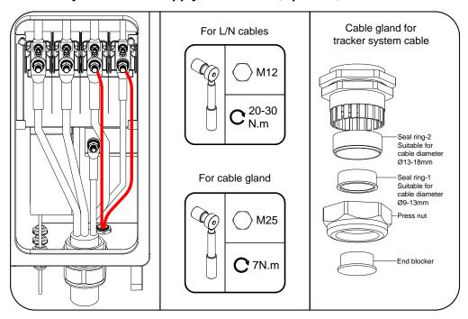
Strip the protection layer and insulation layer by specific length, as described in the figure below.
