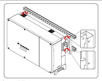
Step 4 Fix the inverter with screws M6x30.
