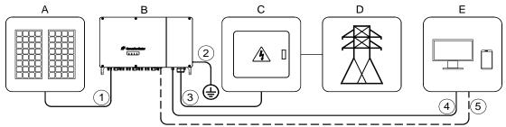
A) PV string; B) Inverter; C) AC distribution box/cabinet; D) Utility grid; E) Monitoring device
