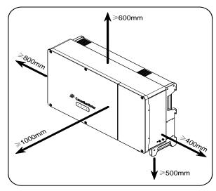
2) In case of multiple inverters, reserve specific clearance between the inverters.
