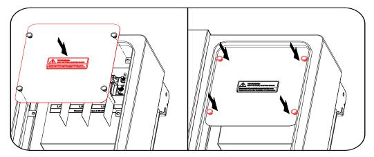
Step 2 Close the wiring compartment and tighten the four screws on its front cover with screwdriver T30.
