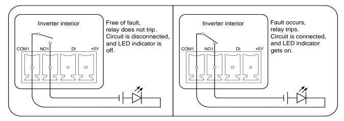
DI terminal (emergency stop dry contact): the dry contact can be configured to be an emergency stop contact. When the DI contact and +5V contact are shorted by external controlled switch, the inverter will immediately stop
