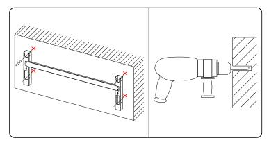
Step 3 Fix the mounting-bracket with the expansion bolts.
