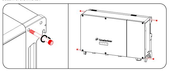
Step 2 Lift and move the inverter to the destination by using the side and bottom handles as well as the four installed hand shanks.
