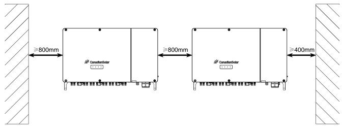
3) In case of back-to-back installation, reserve specific clearance between the two inverters.
