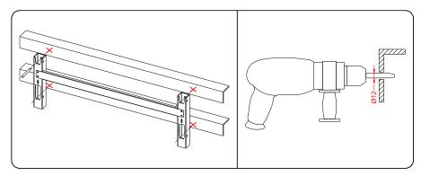
Step 2 Secure the mounting-bracket with M10 bolts and nuts.
