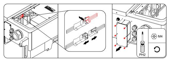
Step 5 Insert the new fan module into the track and secure the screws.
