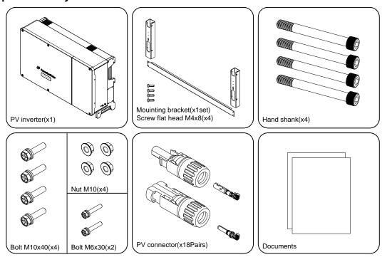
Number of PV connectors, 18 pcs for the type of 9MPPTs, and 12 pcs for the type of 6MPPTs.
