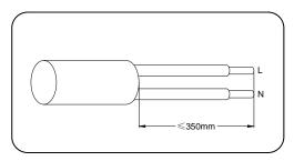
Make the cable and crimp OT/DT/DTM terminal.
