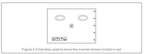
2. Two people are required to remove the inverter from the shipping box. Use the handles integrated into the heat sink to remove the inverter from the carton (see Figure 3.4).
