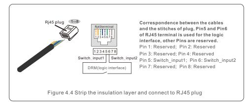
3.Connect RJ45 to DRM (logic interface).
