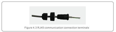
2.Use the network wire stripper to strip the insulation layer of the communication cable. According to the standard line sequence of figure 4.4 connect the wire to the plug of RJ45, and then use a network cable crimping tool to make it tight.
