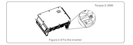
5. Use screws in the packaging to fix the inverter to the mount bracket.
