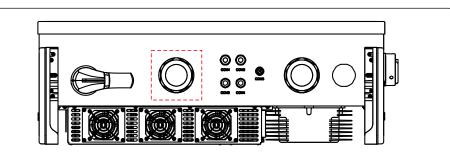
Figure 3.21 Connect the DC Connectors to the Inverter
