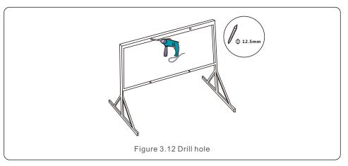
3) Align the mounting plate with the holes, Insert the combination bolt (M10X40)through the mounting plate into the hole. Secure the bracket to the metal frame firmly with the supplied fastener. Torque the nut to 35NM.
