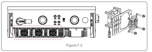
7. Clean or replace the fan. Assemble the fan on the rack.
