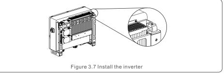
5. Use screws in the packaging to fix the inverter to the mount bracket.
