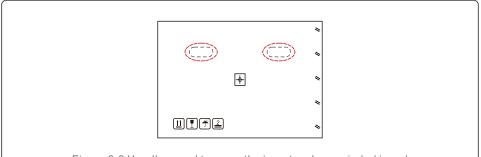
Figure 3.3 Handles used to move the inverter shown circled in red
