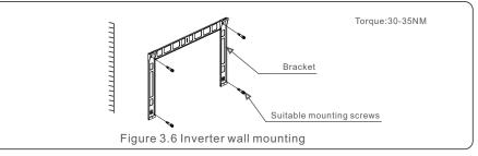
4. Lift the inverter and hang it on the bracket, and then slide down to make sure they match perfectly.
