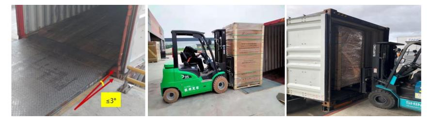
Container bottom level and the loading/ unloading platform level must be at the same level, and the inclination angle must be  $\leq 3^{\circ}$ .
