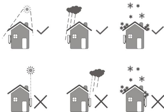
FIG.6-1 Inverter Installation Positions
