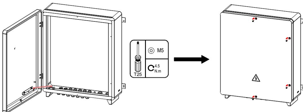
Figure 11 Door Closing Schematic Diagram
