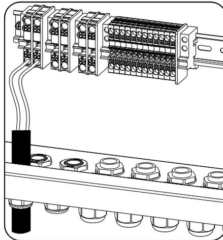
Figure 6 Three-phase AC Line Wiring Diagram
