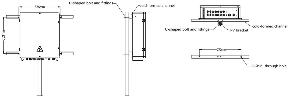
Figure 3 Pole Installation / PV Bracket Installation Schematic Diagram (unit: mm)
