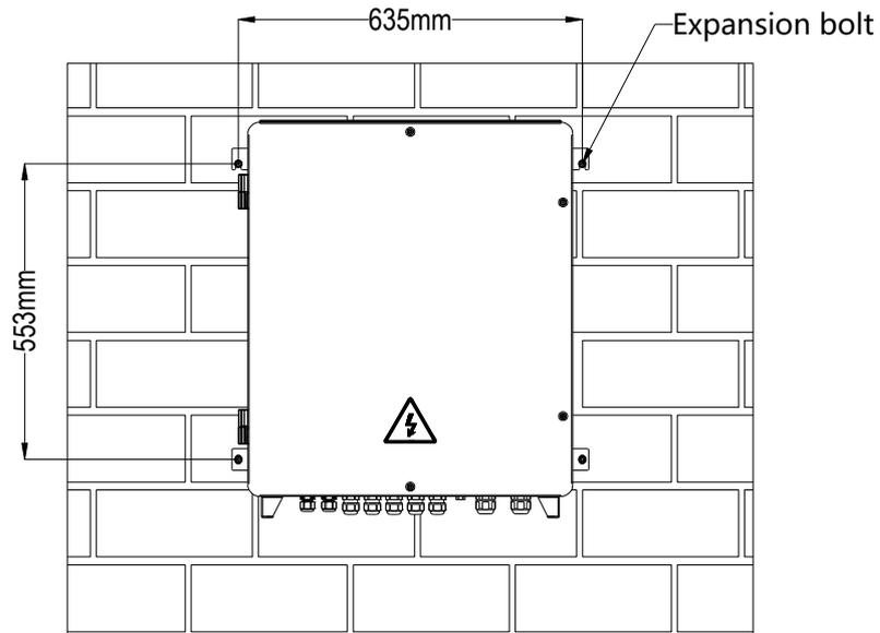
Figure 2 Wall Hanging Installation Schematic Diagram (unit: mm)
