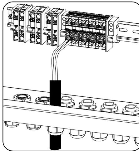
Figure 9 RS485 Line Connection Schematic Diagram
