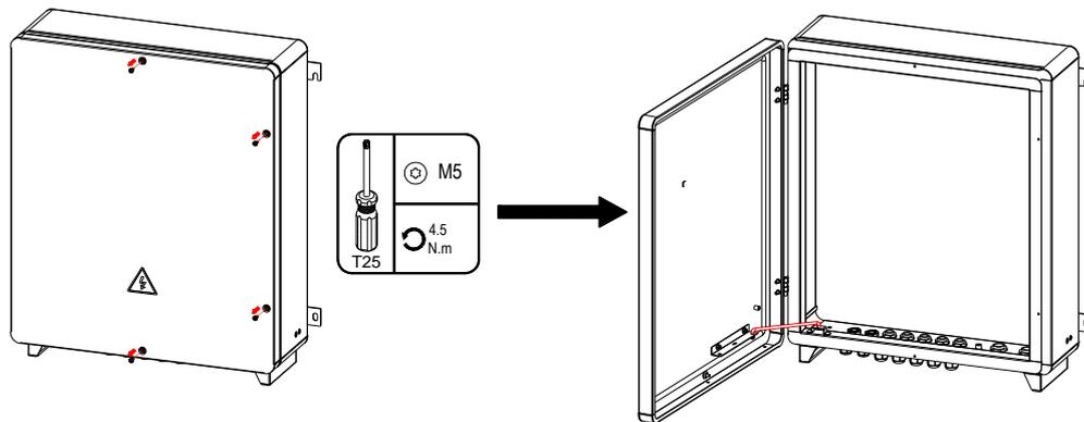
Figure 4 Door Opening Schematic Diagram
