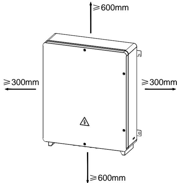
Figure 1 Spatial Distance Schematic Diagram (unit: mm)
