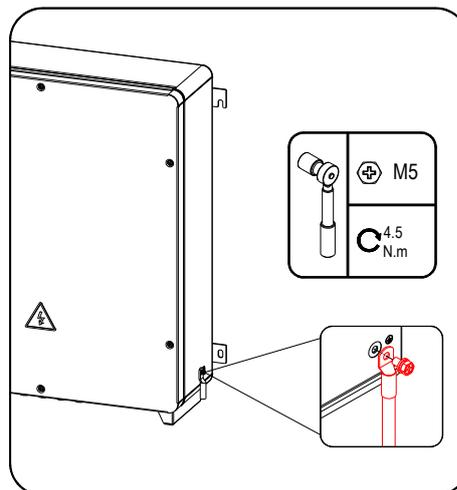
Figure 8 External Ground Wire Connection Schematic Diagram
