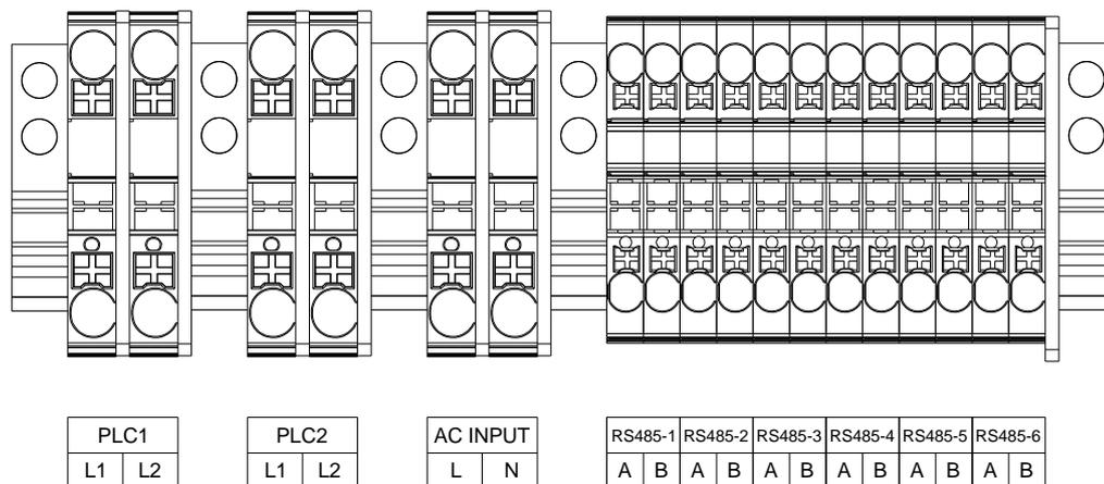
Figure 5 Wiring Port Schematic Diagram
