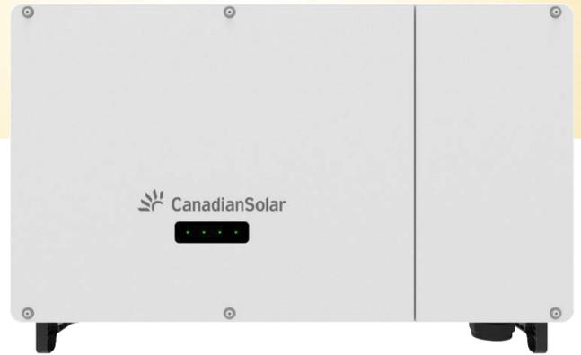
CSI Solar's grid-tied, transformer-less string inverters help to accelerate the use of three-phase string architecture for industrial and commercial rooftop applications. These inverters are modular design building blocks that provide high yield and enable significant BoS cost savings. They provide up to 98.4% conversion efficiency, a wide operating range of 200-1000 V<sub>DC</sub>, and multi choice MPPTs for maximum energy harvesting.
