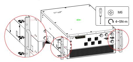
Figure 3-6 Install the fasten parts
