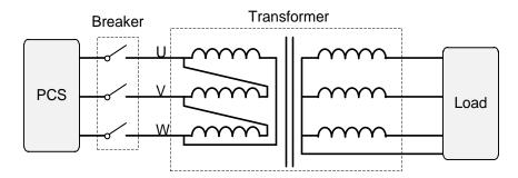
Figure 3-16 Connection diagram (off-grid mode)
