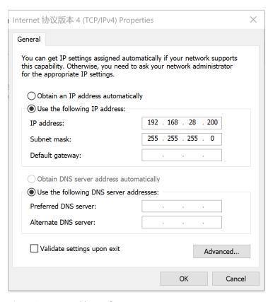
Figure 4-1 Set IP address of computer
