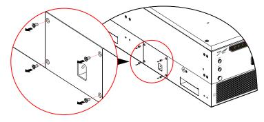
Figure 6-1 Loosen the screws of fan cover
