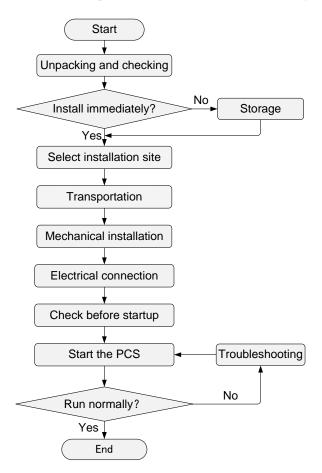
Figure 3-1 Installation process
