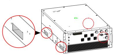
Figure 3-5 Groove position
