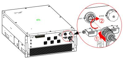
Figure 3-31 ETH port connection diagram
