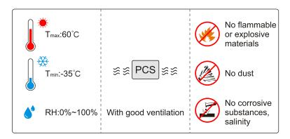
Figure 3-3 Installation environment requirements
