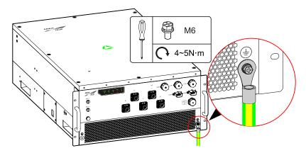
Figure 3-13 Grounding connection diagram
