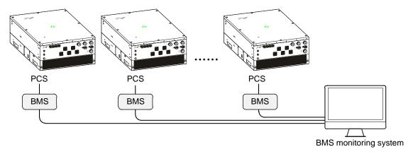
Figure 2-12 Communication with BMS (multiple PCSs)
