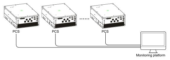
Figure 2-10 Monitoring via Ethernet (multiple PCSs)
