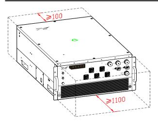
Figure 3-4 Installation Space (unit: mm)
