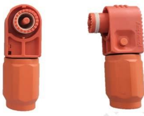
Figure 31: Battery cable quick connect. To install, push into receptacle/terminal until a notable click is heard. To release, press button on side and remove.
