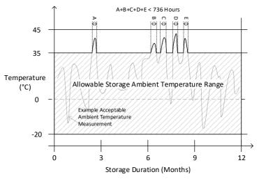
Figure 13- Storage Condition Temperature Limitations
