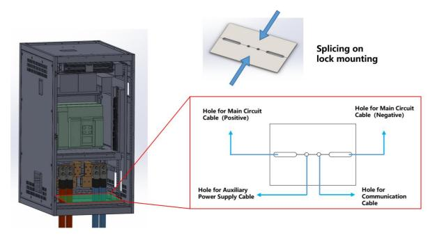
*Figure 9: Location of power cable foundation exit*
