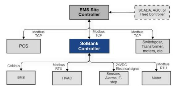
Figure 11: Example ESS communication network with a single SolBank. Site specific network design may vary.
