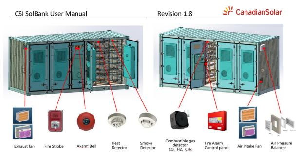
Figure 2: Layout and features of the SolBank
