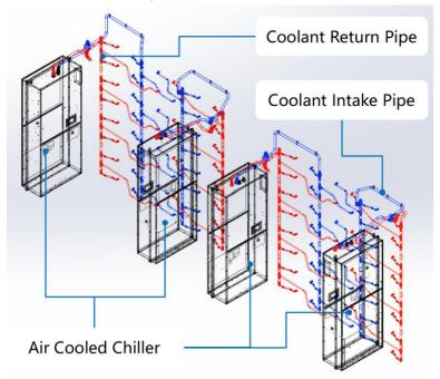
Figure 7: SolBank liquid cooling system schematic
